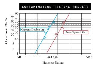
load-life durability tests, environmental tests and millions of in-vehicle test miles. Results of our contamination testing have shown over a 50% increase in life over the current product.
